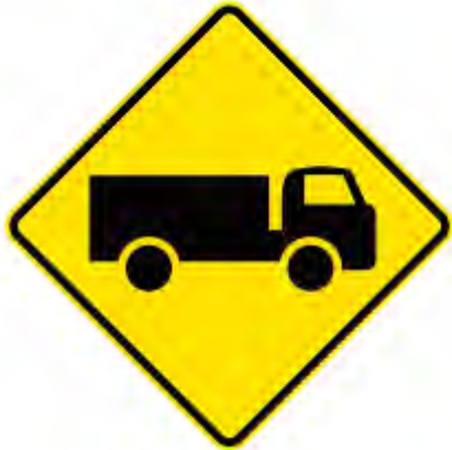
Figure 5-3 W5-22 truck warning signage
