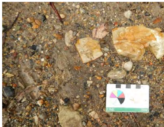
cobble in imported road base at RVRT AC 2
