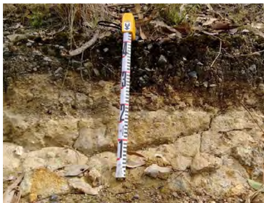
Figure 82: Strata of rail ballast overlying soil and conglomerate layers, north aspect
