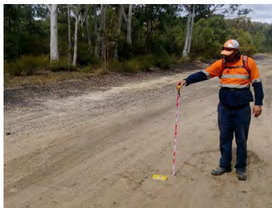
Figure 173: Sandy soil located in erosional ground exposure near base of embankment. South aspect.
