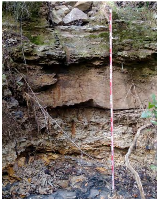
Figure 73: Shale, sandstone and conglomerate strata of Newcastle Coal Measures visible in rail cutting, east aspect
